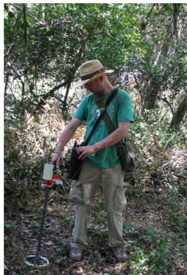
James Adcock using the magnetic susceptibility coil at Vumba
