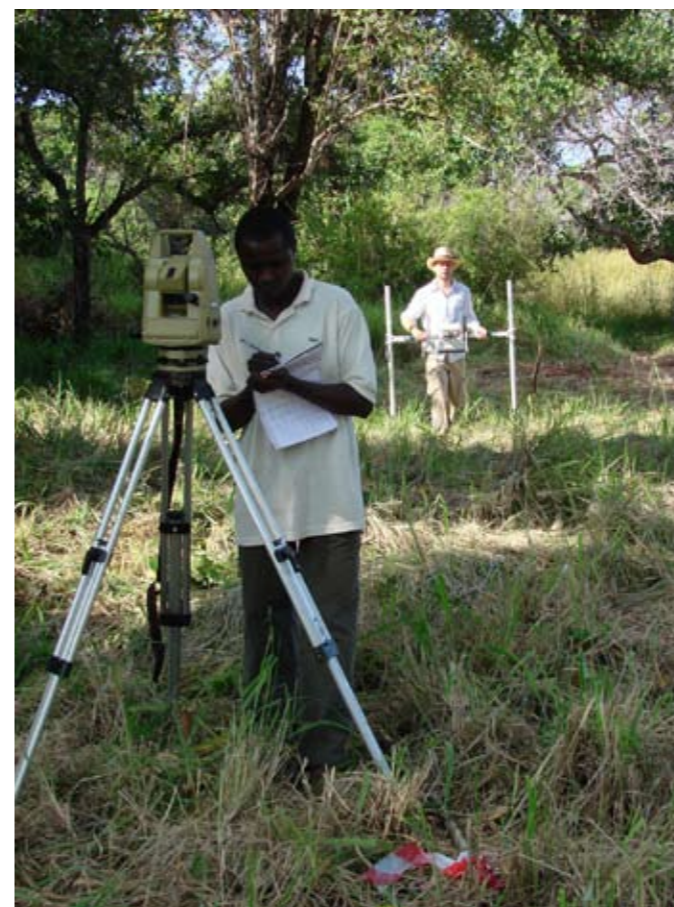
Benson Kimeu uses the EDM total station to map Vumba Kuu. Benson's recent appointment at BIEA greatly enhances our surveying and GIS mapping capabilities and we look forward to offering a much wider range of mapping facilities in the near future.
